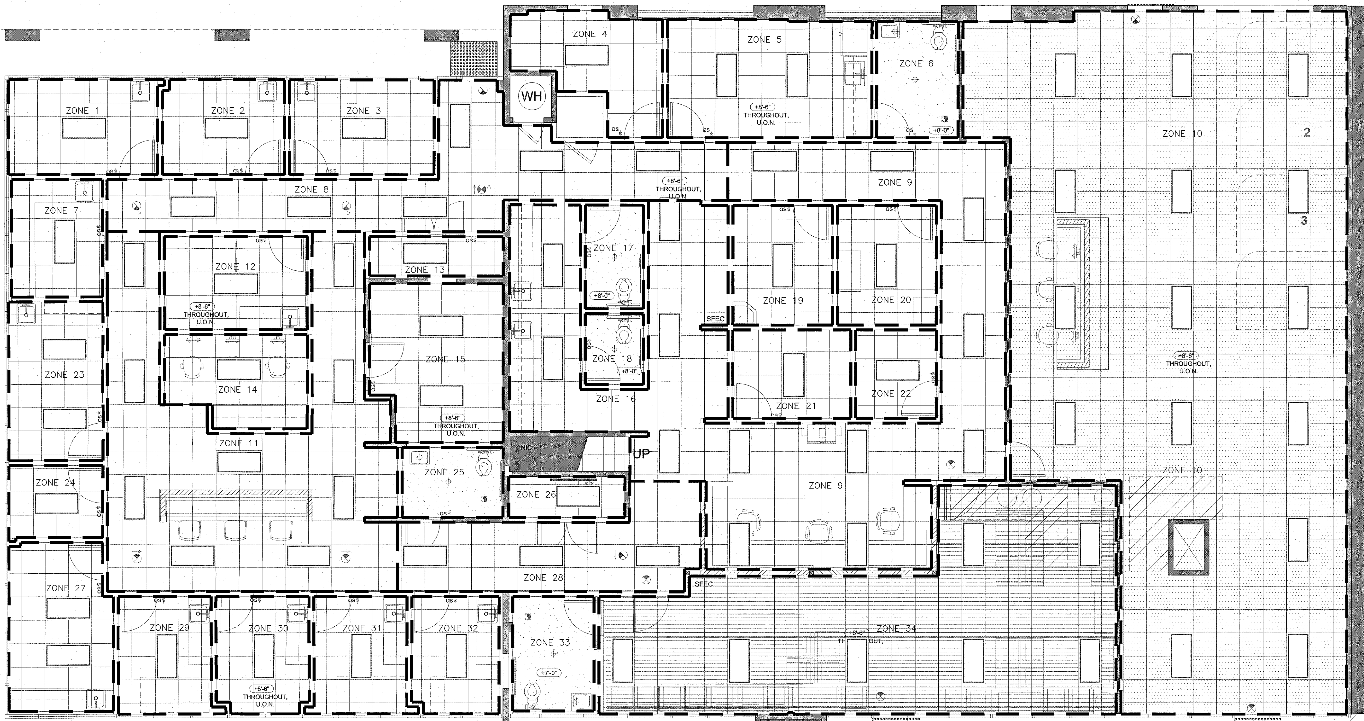
ELECTRICAL LIGHTING ZONES SCALE: 3/16"=1'-0"
